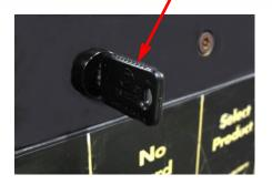
For Turbine, locks are to be installed with the orientation indicator up as shown.
