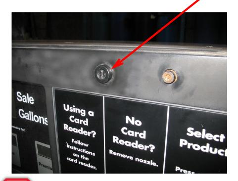
For TuBAR, locks are to be installed with the key ridges upward as shown.
