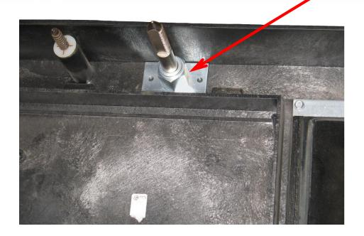
12) Install Mounting Plate (F), Steel Stud(C) and Steel Nut (B). Tighten Nut securely. Steel Stud should have slight "wobble" after nut is securely tightened.
