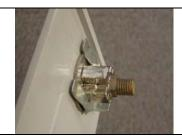
**8.** Loosely remount the old lock's cam on the new lock. Hand start the new nut provided with the new lock on the exposed threads. The nut may only allow a partial turn on the threads by hand. **Warning**: Make sure to only use the new nut provided with the new lock. It has a different thread than the old nut.
