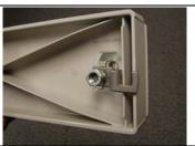
9. Tighten down the nut until the cam is completely seated. Note: It is strongly recommended that while applying torque to the nut that the cam be prevented from rotating. This can be done by either holding the cam approximately as shown or, for some flat doors, clamping a vise grip to the door directly below the cam to prevent excessive internal loads on the lock components. Note: The lock's key can be installed while the nut is being tightened but it is not recommended.
