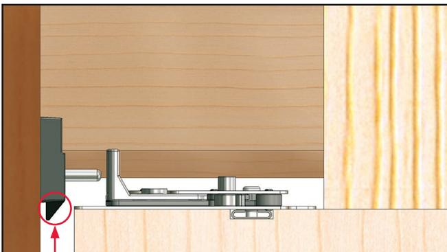
Assure-Sync feature keeps the lock and actuator position synchronized. Low profile pin cam keeps lock from interfering with the drawer box.
