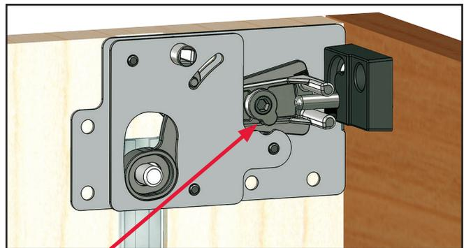
Lock arm adjusts vertically +/- 3/16" for ease of alignment. Lock arm adjusts with 5/32" hex wrench. Low profile actuator fits within 1/2" drawer suspension.
