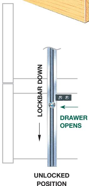
When used with the AP-037 3/8" Adjustable Pin, a strong, rigid lock is provided.
