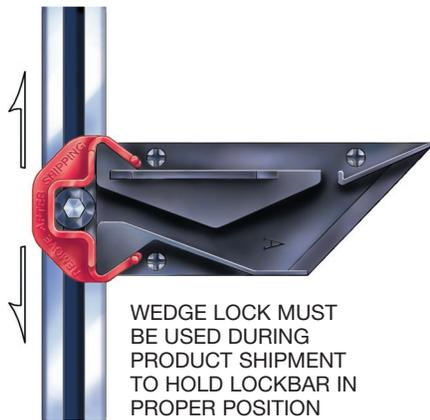
WEDGE LOCK MUST BE USED DURING PRODUCT SHIPMENT TO HOLD LOCKBAR IN PROPER POSITION
