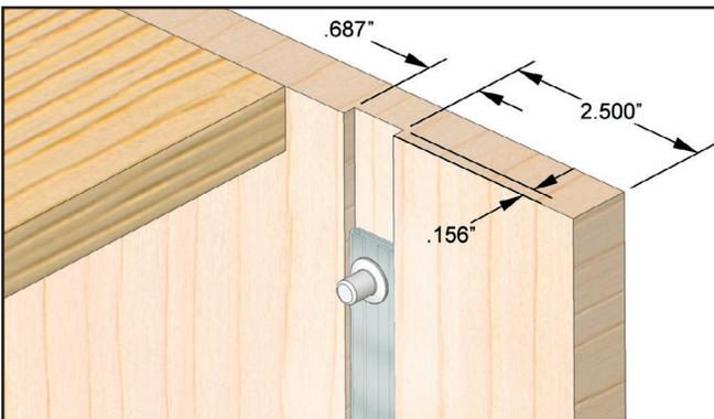
Reference dimensions for end panel with full overlay drawer. Lockbar location is the same for the AC-120 & AC-125 actuators.
