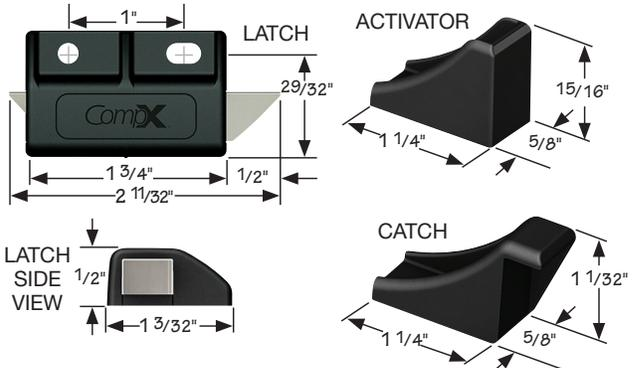
CATCH ON THE SECOND DOOR ACTS AS A SLAM LATCH AND DOES NOT REQUIRE REACHING INTO THE CABINET TO RELEASE
