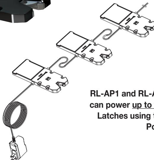
**RL-AP1 and RL-APC-9VJ-10 can power up to 10 Receiver Latches using the RL-APC Power Cords.**
