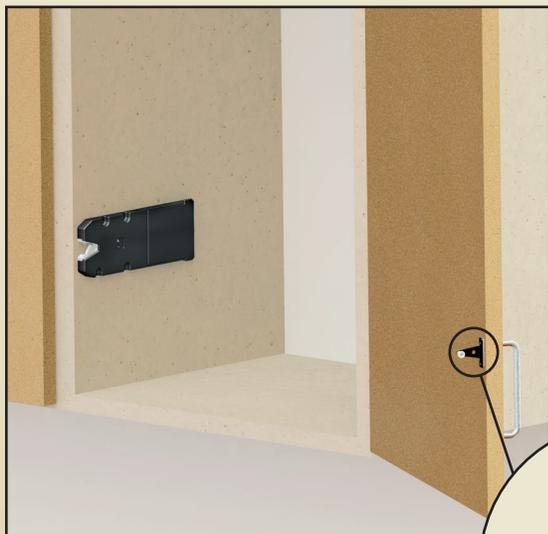
The **Strike Plate** is mounted on the door or drawer to be locked and interfaces with the Receiver Latch.
