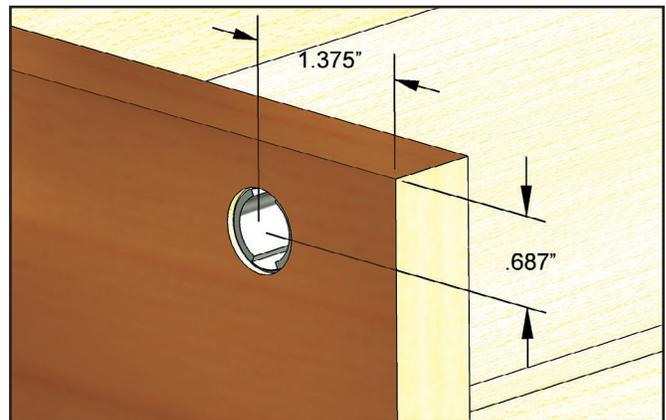
Reference dimensions for lock hole with full overlay drawer and 3/4" end panel.
