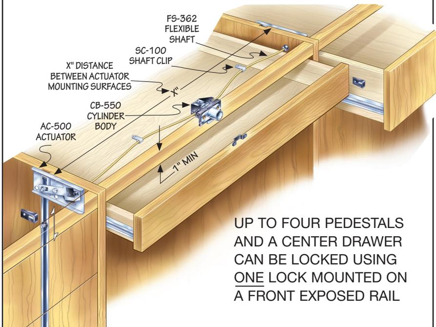
UP TO FOUR PEDESTALS AND A CENTER DRAWER CAN BE LOCKED USING ONE LOCK MOUNTED ON A FRONT EXPOSED RAIL
