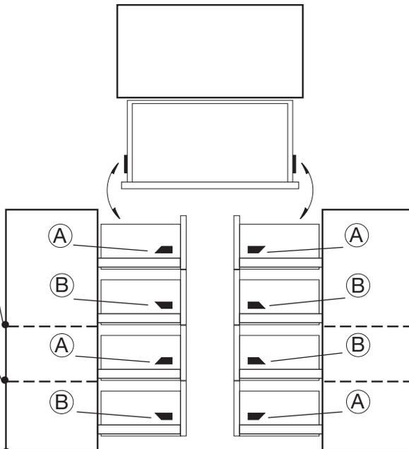
WHEN WEDGES ARE INSTALLED IN THE PROPER POSITIONS AS SHOWN ABOVE, ONLY ONE DRAWER MAY EVER BE OPEN AT ANY ONE TIME... EVEN IF TWO DRAWERS ARE PULLED AT EXACTLY THE SAME TIME!
