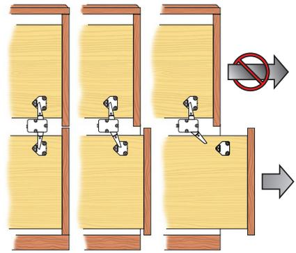
WHEN EITHER DRAWER IS PULLED OPEN, THE DRAWER CLIP ON THAT DRAWER MOVES THE SNAPPER INTO A LOCKED POSITION. THIS PREVENTS ANY FURTHER DRAWERS FROM BEING OPENED.
