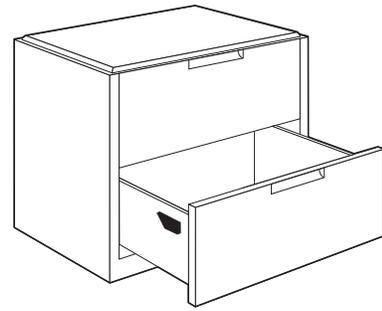
WHEN ANY DRAWER IS PULLED OPEN, THE WEDGES ON THAT DRAWER MOVE THE LOCKBAR INTO A LOCKED POSITION... THEREBY PREVENTING ANY FURTHER DRAWERS FROM BEING OPENED
