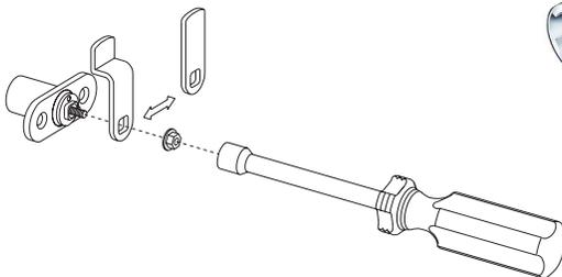
THE 'THICK PANEL LOCK' COMES PACKAGED WITH 2 DIFFERENT CAMS WHICH CAN BE ASSEMBLED TO THE LOCK IN ANY OF THE 3 ORIENTATIONS ILLUSTRATED TO THE RIGHT. THIS OFFERS SUFFICIENT FLEXIBILITY TO ADAPT TO MOST LOCKING SITUATIONS.
