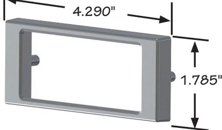
Mounting screws fit material 5/8" - 7/8" thick
