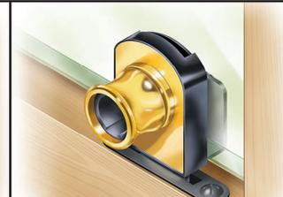
**CAM MUST ROTATE COUNTER-CLOCKWISE TO LOCK**
