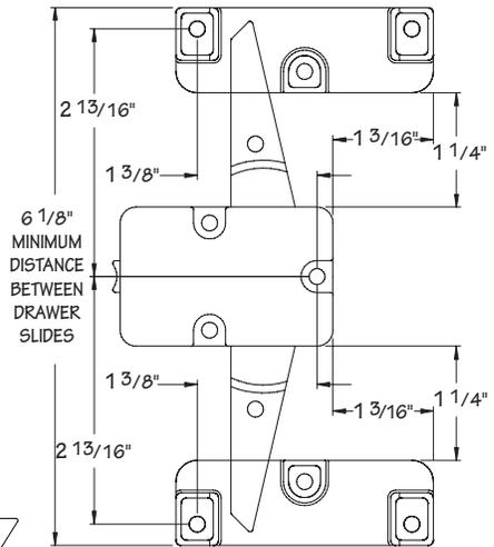
LINKAGE BAR FOR THREE OR FOUR DRAWER APPLICATIONS DC-400 SHOWN
