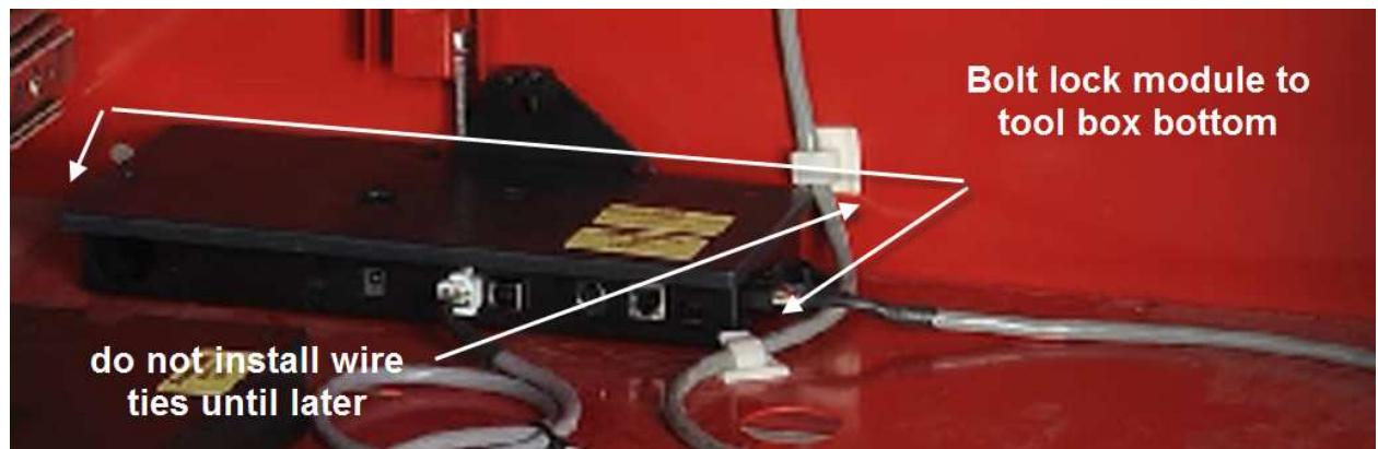
9. Next we're going to install the cables into the electronic lock module. The main cable originating in the proximity faceplate plugs into the right side of the electronic lock module. Align the tab on the top of the connector with the locking clip on the cable connector.
