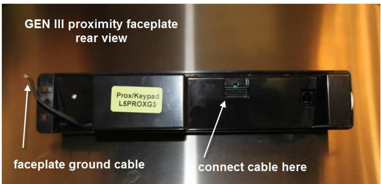
Connect the cable to the rear of the faceplate aligning the top of the cable connector clip.
