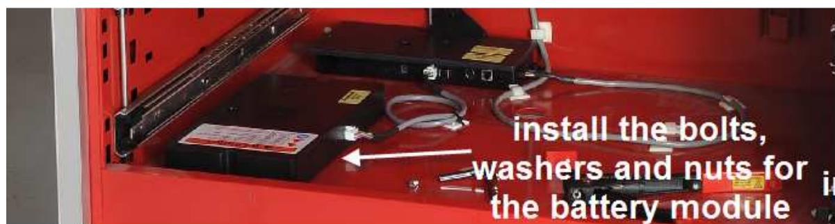
Be sure you have all necessary wires installed and plug-in to their modules prior to tying any wires in place
