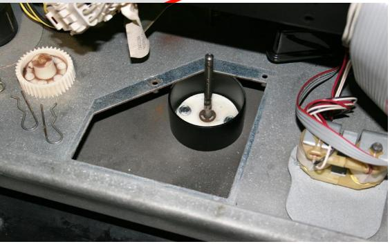
from the underside, install one screw (H) thru Drive Shaft Assembly, lower panel and into one hole of the Lower Pulser Security Sleeve. DO NOT tighten screw. Rotate Lower Pulser Sleeve to line up second hole with the lower panel and install second Screw (H). Tighten both screws. Complete installation by installing Totalizer Security Cover Kit.
