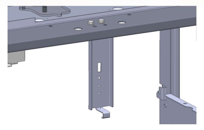
16. Drill Ø3/8" holes in both sides of the frame in the approximate location shown.
