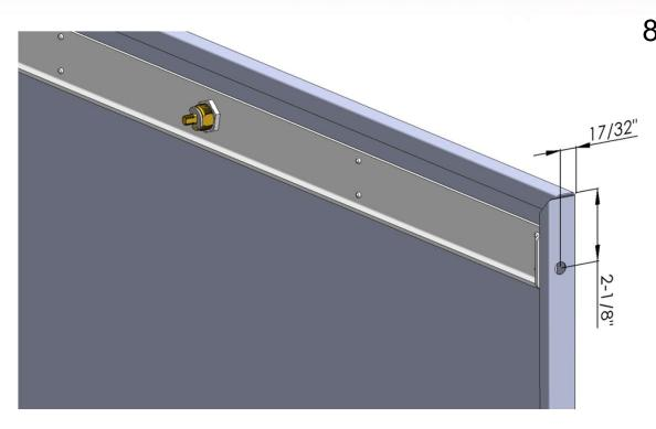
5. Drill (2) Ø3/8" holes in both sides of Door Panel in the approximate location shown from top and front faces.
