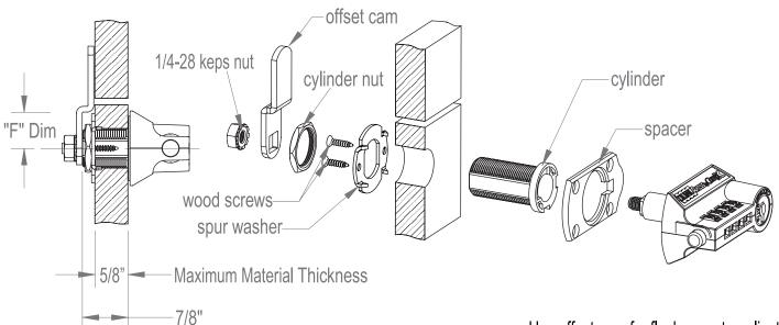
Use offset cam for flush mount applications
