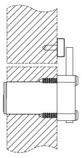
Lock is shown in locked position for standard drawer applications.
