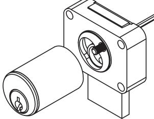
Use a 5/64" Allen wrench from the back to remove the cylinder.
