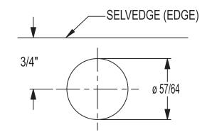
DRILL 1/16 INCH DIAMETER PILOT HOLES FOR MOUNTING SCREWS
