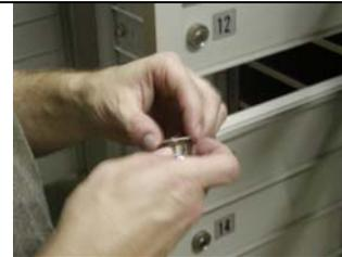
**5. Peel off the liner** from the washer exposing the adhesive.
