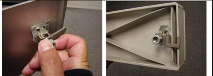
**9. Tighten down the nut** until the cam is completely seated. Note: It is strongly recommended that while applying torque to the nut that the cam be prevented from rotating. This can be done by either holding the cam approximately as shown or, for some flat doors, clamping a vise grip to the door directly below the cam to prevent excessive internal loads on the lock components. Note: The lock's key can be installed while the nut is being tightened but it is not recommended.
