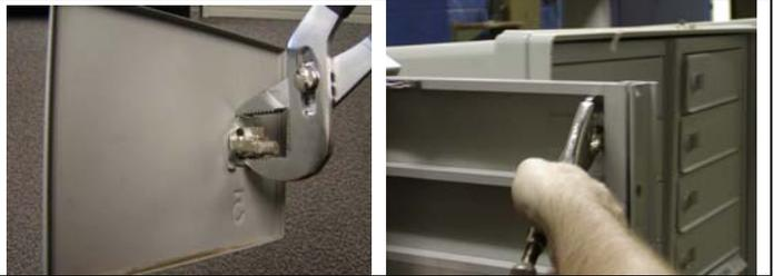
**7b. Shim spacing is needed if** the spring clip installed easily but is not securing the lock to the door adequately or if the spring clip is too tight to squeeze into place. In this case, use additional washers on the backside of the door to fill the gap so that the spring clip can secure the lock to the door using the back set of grooves.
